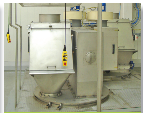
Bag emptying pad filter
