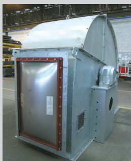
Explosion vent at elevator head
